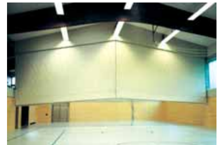
Inclined curtain hoist systems for halls with gable or pent roof.
