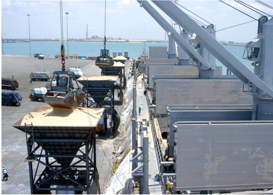
Unloading Raw Sugar from Vessel using cranes and loading into the hopper
