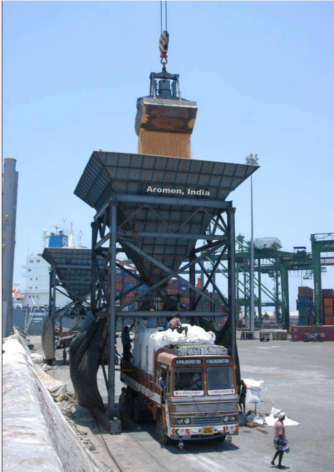
Side view of Portable Hopper (Tutocorin Port, India)
